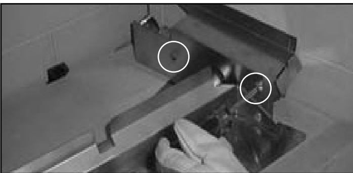
Figure 11.2 Remove Pilot Shield
